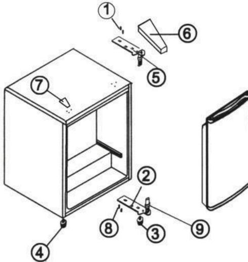
Remove the upper hinge cover (6) screws (1) and hinge (5)
